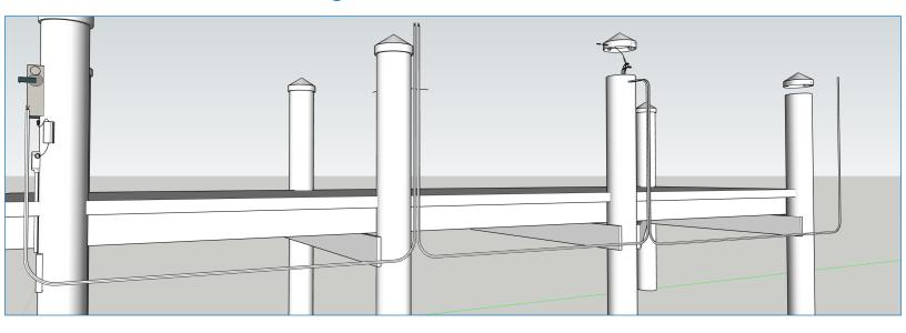
Each U-shape extension wire is tailored, threaded and stapled under dock deck or behind structures
