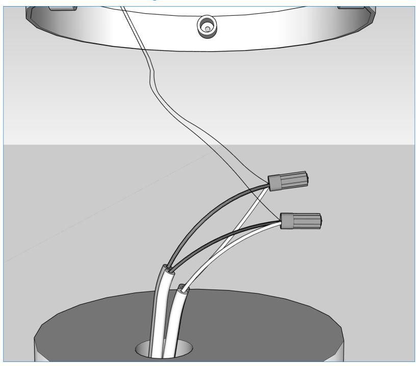
In connections, connect multiple positive conductors together and multiple negative conductors together. If connect incorrectly lights will not light up but will not break either; then re-connect them correctly.
